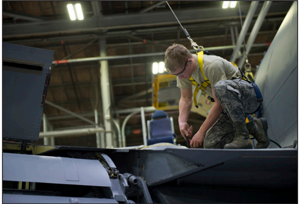
Airman 1st Class Noah Stancik, 434th Maintenance Squadron aircraft mechanic, removes panels from the wing of a KC-135R Stratotanker at Grissom March 1.
